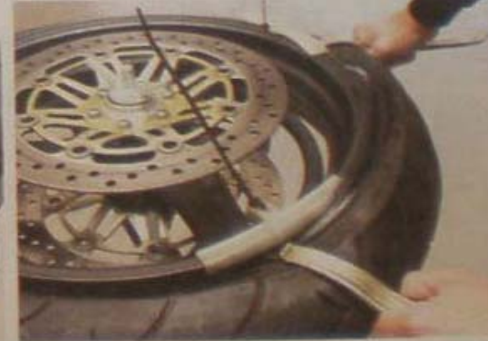
With the final bites of your tire irons, the tire popping onto the rim will be your reward. That, and the money you saved!
