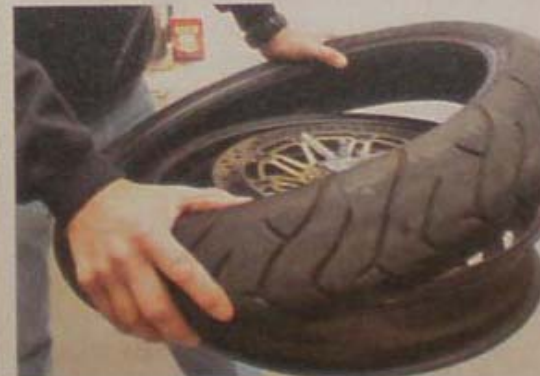
Reinstall by pushing the lower bead over the rim. Check directional arrows and align painted dots with the valve stem.
