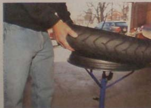
Once the first bead is released, it's fairly easy to get the next one free. The rim's drop center provides extra clearance.
