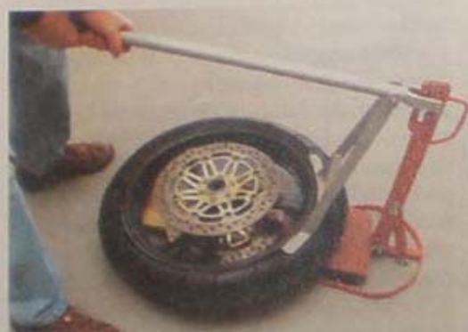
My handy JC Whitney bead breaker works on both car and bike tires (use blocks).
