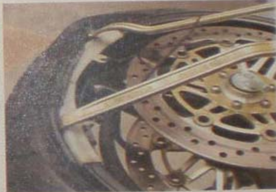
Long tire irons give better leverage, and rim protectors will prevent scratches.
